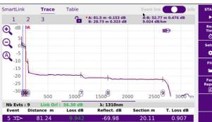
FTTH-SLM (SmartLink Mapper) is an OTDR software application dedicated to FTTH/PON OTDR testing, to characterize each section of the network as well as passive components such as splitters, connectors and splices. It dynamically adjusts the testing parameters and automatically performs multiple measurements to achieve the optimum test results. All the information gathered is displayed as a single icon-based view and a combined OTDR trace.
